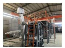
The machine is equipped with an integrated work platform to facilitate demoulding & charging and improve work efficiency.
