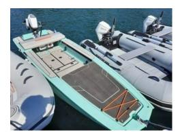
Marketed by the Brunswick Group, the Veer brand offers rotomolded polyethylene canoes for fishing or cruising. Designed for protected waters, the Veer X13 is a 4-meter boat that displaces 180 kg. Made from rotomolded polyethylene, it is approved for two passengers.
