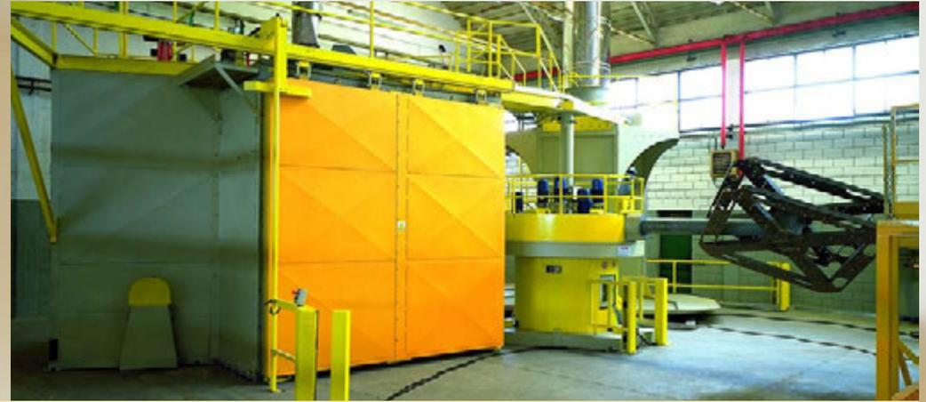
*The arms move all together and alternate in the production phases at the same time. It can be configured with a cooling chamber and with 2, 3 or 4 interchangeable mold holder arms, choosing straight arms to produce groups of molds or angled arms for larger rotomoulded products according to specific needs.*
