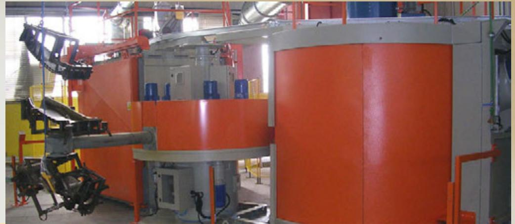
*Given the duration of the critical phase of the process, which can be the formation of the shot in the rotational molding oven, the cooling and extraction phase of the piece, the shots alternate with the same cadence as the arms move from one phase to another simultaneously.*
