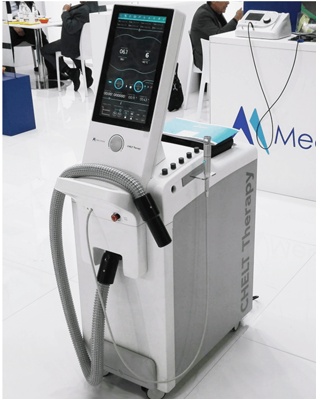
> The main body is made through rotational technology
