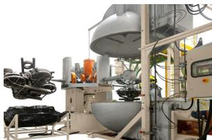
Rotational molding machines usually have doors, but the Sphere Oven SO 1.60 opens and closes vertically, which enables a more homogenous air flow, reduces heat loss and saves space, according to Rotoline Industrial Equipment Ltda. Rotoline Industrial Equipment Ltda. has introduced
