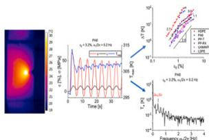
To investigate intrinsic heating and thermoelastic coupling separately, static tension and dynamic deformation controlled fatigue tests at  $\omega_1/2\pi = 0.2$  Hz and 5 Hz were performed for six polymers: high density polyethylene (HDPE), low density polyethylene (LDPE), ultra high molecular weight polyethylene (UHMWPE), polyamide 6 (PA6) and two grades of polypropylene (PP); i.e. an injection grade (PP-T) and a rotomolding grade (PP-RX).
