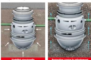
This oil or grease separator is made of rotomolded polyethylene. The tanks have an egg-shaped bottom and a wall thickness of 10mm. The shape as well as the robust execution of the tank guarantee structural stability and allow maximum mechanical resistance, making it possible to install into closing devices in class A and B without a distribution slab, and in class D with a distribution ring directly applied to the compacted soil.
