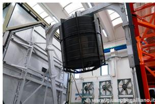
Polivinil Rotomachinery is a well known Italian manufacturer of rotational molding equipment. Its latest offering, the SRM-7500 machine is the world's largest double trolley shuttle for rotomolding ever. It comes equipped with large robotic arms that are long enough to operate in an action space of up to 7500mm. (Translated from Italian)
